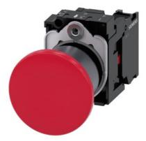
Mushroom pushbutton, 22 mm, round, plastic with metal front ring, red, 40mm, latching, pull-to-unlatch mechanism, with holder, 1 NC, screw terminal, with laser labeling, lower case
