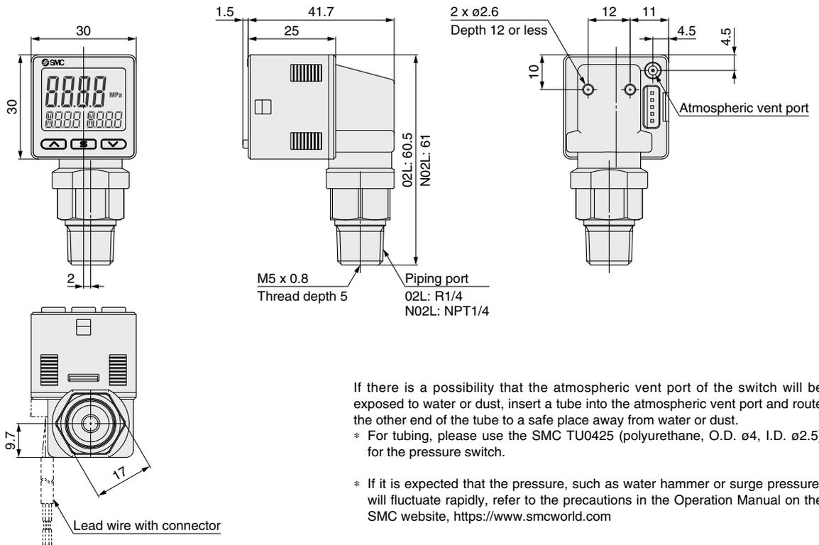
If there is a possibility that the atmospheric vent port of the switch will be exposed to water or dust, insert a tube into the atmospheric vent port and route the other end of the tube to a safe place away from water or dust.
