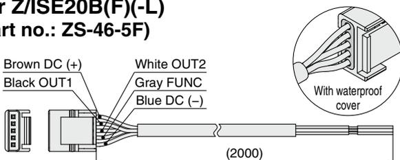
\* For the lead wire with M12 connector, refer to page 39.
