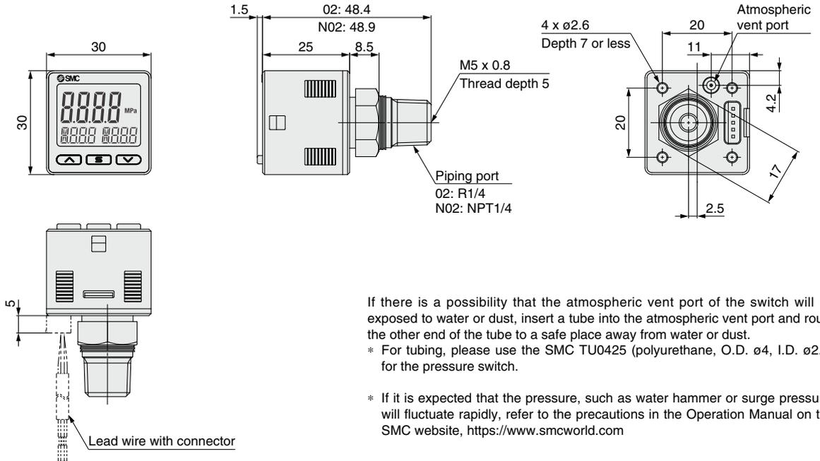
If there is a possibility that the atmospheric vent port of the switch will be exposed to water or dust, insert a tube into the atmospheric vent port and route the other end of the tube to a safe place away from water or dust.
