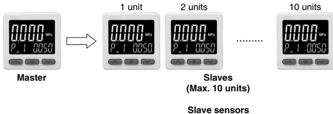
\* This function is not provided with the IO-Link compatible type.
