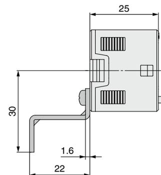
\* When using the bracket B, install it by taking the dimensions of the piping part into consideration.
