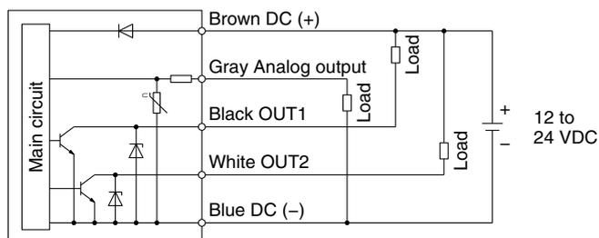
**-T: PNP (2 outputs) + Analog voltage output**
