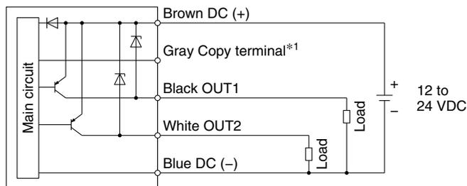
**-R: NPN (2 outputs) + Analog voltage output**
