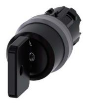
Key-operated switch O.M.R, 22 mm, round, plastic with metal front ring, lock number 73034, black, with 2 keys, 3 switch positions I-O-II, left latching, right momentary contact type, actuating angle  $2x45^{\circ}$ , 10:30h/12h/13:30h, key removal I, with laser labeling, upper case
