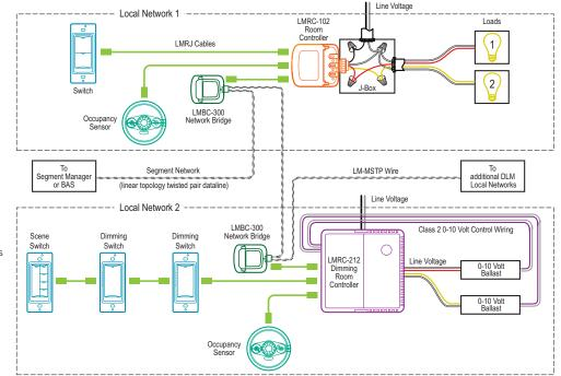
Plug DLM local network components together in any configuration using Cat 5e cables with RJ45 connectors.
