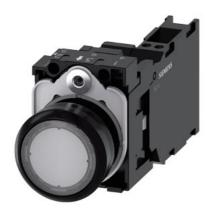
Illuminated pushbutton, 22 mm, round, plastic, clear, pushbutton, flat, momentary contact type, with holder, 1 NO+1 NC, LED module with integrated LED 24 V AC/DC, spring-type terminal, with laser labeling, upper case
