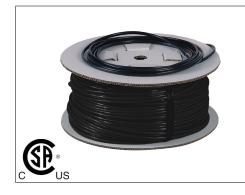
Danfoss TX-FH cables are a thick floor heating solution. Thick cables have a larger diameter than the Danfoss LX Floor Heating cables, allowing them to be lower in COST, higher in HEAT OUTPUT, and more DURABLE. They are installed in mud beds below the flooring materials and are most often used in new construction where overall material cost is a primary concern.
