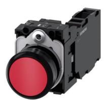
Pushbutton, 22 mm, round, plastic, red, pushbutton, flat, momentary contact type, with holder 1 NO+1 NC, screw terminal, with laser labeling, upper case and lower case, always upper case at beginning of line
