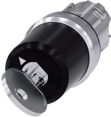
key-operated switch Siemens, 22 mm, round, metal, shiny, lock no. STGH10, with 2 keys, 2 switch positions O-I, latching, actuating angle 90°, 10:30h/13:30h, key removal O+I, Z=50-unit packaging
