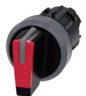
Selector switch, illuminable, 22 mm, round, plastic with metal front ring, red, selector switch, short, 3 switch positions I-O<II, left latching, right momentary contact type, actuating angle  $2x45^{\circ}$ , 10:30h/12h/13:30h, with laser labeling, lower case
