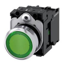
Illuminated pushbutton, 22 mm, round, Metal, shiny, green, pushbutton, flat, momentary contact type, with holder, 1NO, LED module with integrated LED 230 V AC, screw terminal, with laser labeling, symbol number according to, ISO 7000 or IFC 60417
