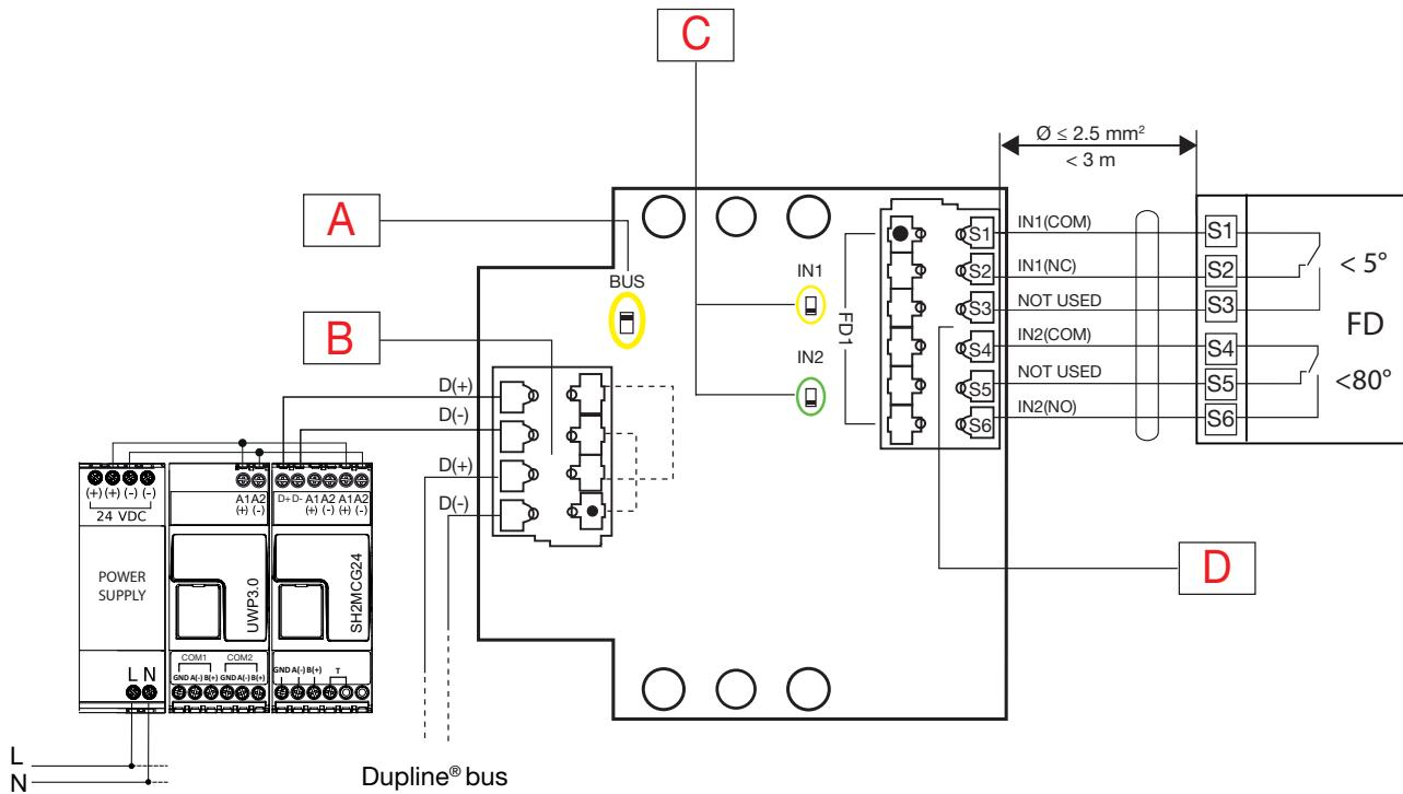
**Fig. 1 Example of a fire damper connection**
