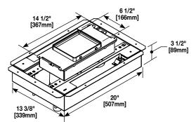
Fire Classified Two-Compartment Box – For use in either concrete or wood floors. Fully adjustable with tunnel compartment. Supplied with one (1) duplex receptacle, mounting plate, and one (1) communication mounting plate (RFB22AB). Other device plates sold separately.
