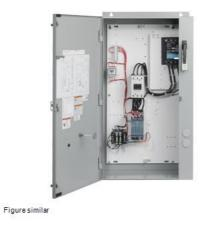
Enclosed soft starter, Controller 3RW40766BB34, Std duty rating 125HP @200V, Std duty current rating 385A Control voltage 115Vac Combination type, 600Amp fusible disconnect, Enclosure type NEMA 3/3R Weather proof outdoor use
