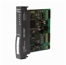
The GDP-N gateway serves to connect the *excom*® system to PROFIBUS-DP networks. Connection to the PROFIBUS-DP is established via optical fibers or copper cables. When using optical fibers for data transmission, an optocoupler pair must be installed between wired and optical PROFIBUS.
