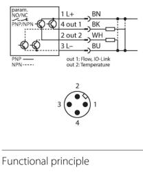
The flow sensor functions according to the calorimetric principle. The distinctive feature of this principle is that the flow rate correlates directly to the thermal loss of energy in the probe. The increased loss of energy is
