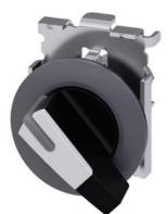
Selector switch, illuminable, 30 mm, round, Metal, matte, white, selector switch, long, front ring for flush installation, 2 switch positions O-I, latching, actuating angle 90°, 10:30h/13:30h, with laser labeling, upper case and lower case, always upper case at the beginning of the word
