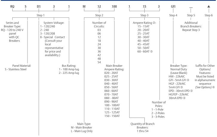
@ Panel Size: Select A1, B1, C1, D1, J1, F1, L1 or H1 stainless steel enclosure based on number of circuits
