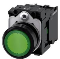
Illuminated pushbutton, 22 mm, round, plastic, green, pushbutton, flat, momentary contact type, with holder, 1NO, LED module with integrated LED 230 V AC, screw terminal, with laser labeling, upper case and lower case, always upper case at beginning of line
