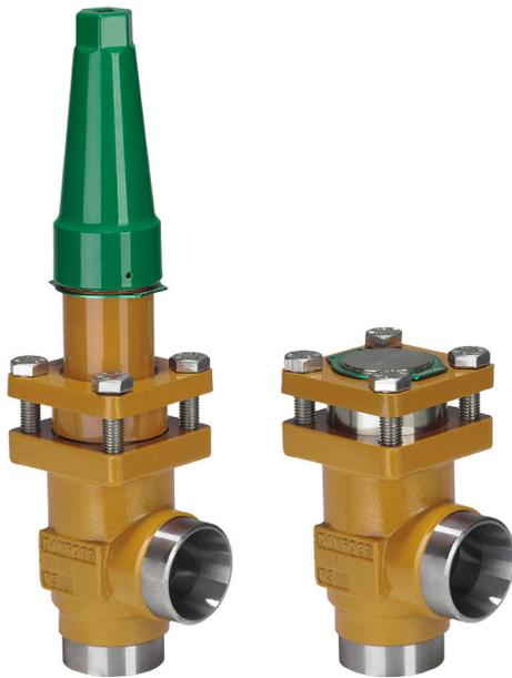
SCA-X are check valves with a built-in stop valve function. CHV-X are check valves only. SCA-X/ CHV-X are available in angleway and straightway versions. The valves are designed to open at very low differential pressures, allow favourable flow conditions and are easy to disassemble for inspection and service.
