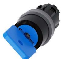
Key-operated switch O.M.R, 22 mm, round, plastic with metal front ring, lock number 73038, blue, with 2 keys, 2 switch positions O-I, latching, actuating angle 90°, 10:30h/13:30h, key removal O, with laser labeling, lower case
