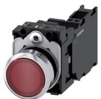
Illuminated pushbutton, 22 mm, round, metal, shiny, red, pushbutton, flat, momentary contact type, with holder, 1 NO+1 NC, LED module with integrated LED 24 V AC/DC, spring-type terminal, with laser labeling, symbol number according to, ISO 7000 or IEC 60417
