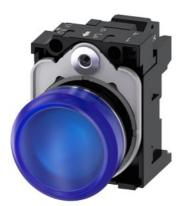
Indicator lights, 22 mm, round, metal, shiny, blue, lens, smooth, with holder, LED module with integrated LED 110 V AC, spring-type terminal, Z=20-unit packaging
