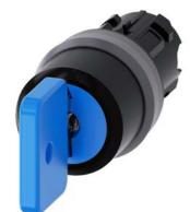
Key-operated switch O.M.R, 22 mm, round, plastic with metal front ring, lock number 73038, blue, with 2 keys, 3 switch positions I-O<II, left latching, right momentary contact type, actuating angle 2x45°, 10:30h/12h/13:30h, key removal O, with laser labeling, upper case and lower case, always upper case at beginning of line
