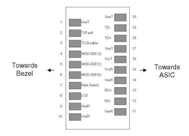
Pin-out of connector Block on Host board
