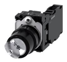
RONIS key-operated switch, 22 mm, round, plastic, lock number SB30, with 2 keys, 2 switch positions O-I, latching, 10:30h/13:30h, key removal O+I, with holder, 1 NO+1 NC, screw terminal, possible special locks: SB31, 421, 455, with laser labeling, upper case
