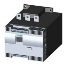
SIRIUS soft starter Values at 400 V, 40 °C standard: 432 A, 250 kW Inside-delta: 748 A, 400 kW 200-460 V AC, 230 V AC Screw terminals !!! Phased-out product !!! Successor is SIRIUS 3RW5, Preferred successor type is >>3RW5547-6HA14<<
