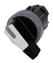
Selector switch, illuminable, 22 mm, round, plastic with metal front ring, white, selector switch, long, 2 switch positions O-I, latching, actuating angle 90°, 10:30h/13:30h, with laser labeling, upper case and lower case, always upper case at beginning of line
