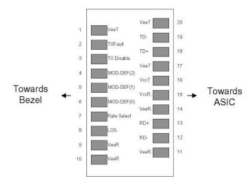
Pin-out of connector Block on Host board
