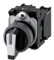
Selector switch, illuminable, 22 mm, round, plastic with metal front ring, white, selector switch, short, 3 switch positions I-O-II, latching, actuating angle 2x45°, 10:30h/12h/13:30h, with holder, 1 NO, 1 NO, screw terminal, with laser labeling, inscription or symbol Customer-specific selection with SIRIUS ACT configurator (CIN)
