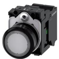
Illuminated pushbutton, 22 mm, round, plastic, clear, pushbutton, flat, momentary contact type, with holder, 1NO, LED module with integrated LED 230 V AC, spring-type terminal, with laser labeling, upper case
