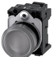
Indicator lights, 22 mm, round, plastic, clear, lens, smooth, with holder, LED module, with integrated LED 24 V AC/DC, spring-type terminal, with laser labeling, lower case
