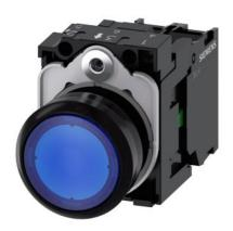
Illuminated pushbutton, 22 mm, round, plastic, blue, pushbutton, flat, momentary contact type, with holder, 1NO, LED module with integrated LED 24 V AC/DC, screw terminal, with laser labeling, symbol number according to, ISO 7000 or IEC 60417
