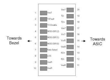
Pin-out of connector Block on Host board
