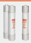
Mersen fuses for the protection of transformers and distribution lines deliver overload and short circuit protection. These current-limiting fuses will melt at current that can be as low as 1.7 times the fuse current ratings up to its maximum interrupting rating. These fuses are designed to withstand the transformer magnetizing inrush current. They have 2 (size C), 3 (size D) and 4 (size E) inch diameter barrels with ferrules and are mounted in spring reinforced clips.
