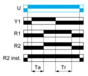
Function B: Single Interval Relay with Control Signal
