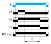
Function D: Symmetrical Flashing Relay (Starting Pulse-Off)
