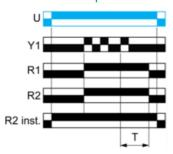
Function O: Delayed Safe-Guard Relay
