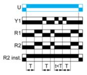
Function P: Pulse Delayed Relay with Fixed Pulse Length
