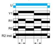
Function C: Off-Delay Relay with Control Signal
