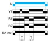
Function Ah: Pulse Delayed Relay (Single Cycle) with Control Signal
