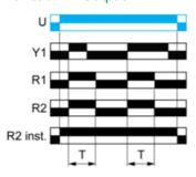
Function Bw: Double Interval Relay with Control Signal
