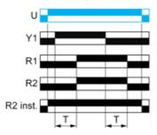
Function Ad: Pulse Delayed Relay with Control Signal
