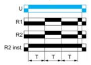
Function Di: Symmetrical Flashing Relay (Starting Pulse-On)
