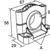
**Hole center spacing:** A=ø 50.8
