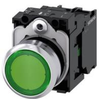
Illuminated pushbutton, 22 mm, round, metal, shiny, green, pushbutton, flat, momentary contact type, with holder, 1NO, LED module with integrated LED 110 V AC, screw terminal, with laser labeling, upper case and lower case, Always upper case at the beginning of the word
