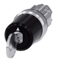
key-operated switch Siemens, 22 mm, round, metal, shiny, lock number SSG10, with 2 keys, 3 switch positions I-O-II, latching, actuating angle 2x45°, 10:30h/12h/13:30h, key removal I, with laser labeling, upper case and lower case, always upper case at the beginning of the word
