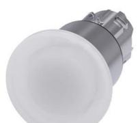
Illuminated mushroom pushbutton, 22 mm, round, metal, shiny, white, 40 mm, 3 switch positions, after pushing in Retraction to center position, after pulling out the button Retraction to center position, with laser labeling, upper case and lower case, always upper case at beginning of line
