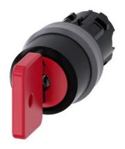
Key-operated switch O.M.R, 22 mm, round, plastic with metal front ring, lock number 73037, red, with 2 keys, 3 switch positions I-O-II, latching, actuating angle 2x45°, 10:30h/12h/13:30h, key removal O, with laser labeling, upper case and lower case, always upper case at the beginning of the word
