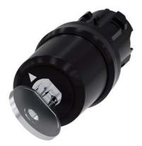
Key-operated switch BKS, 22 mm, round, plastic, Lock No. E2 (VW), without key, 2 switch positions O-I, latching, actuating angle  $90^\circ$ , 10:30h/13:30h, key removal O+I, with laser labeling, lower case
