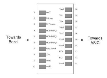
Pin-out of connector Block on Host board
