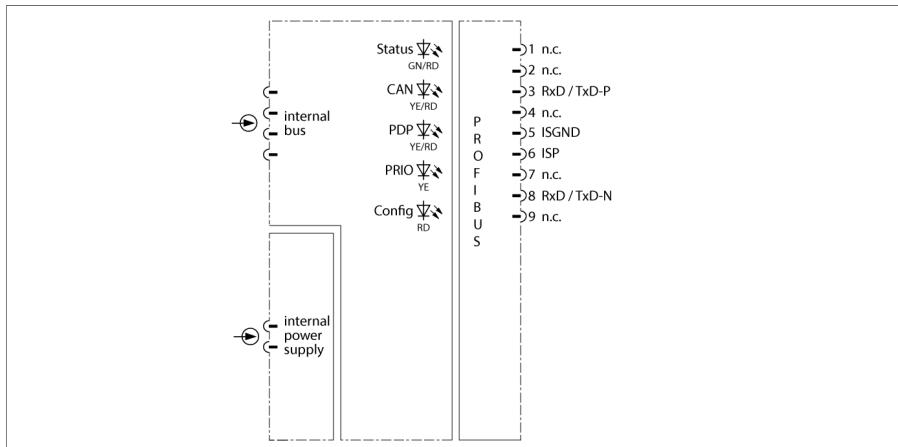
The GDP-IS gateway serves to connect the excom® system to PROFIBUS-DP networks. Connection to the PROFIBUS-DP is established via optical fibers or copper cables. When using optical fibers for data transfer an optocoupler pair must be installed between wired and optical PROFIBUS which also adapts the level to the IS layer. When using copper cables a segment coupler (RS485-IS coupler) must be installed to ensure explosion protection.
