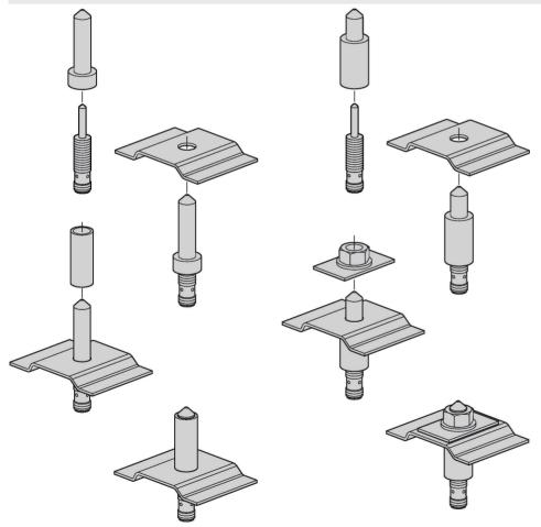
The magnetic field sensor for detection of ferromagnetic spares is especially suited for the detection of welding nuts as well as spacer or reinforcing sleeves. The parts to be detected must always consist of ferromagnetic material, so that a proper function can be guaranteed. Most applications need center bolts to tack
