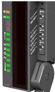
Figure 52. DIP switch configuration to enable cascade installation
