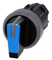
Selector switch, illuminable, 22 mm, round, plastic with metal front ring, blue, selector switch, short, 3 switch positions I-O-II, latching, actuating angle 2x45°, 10:30h/12h/13:30h, Z=50-unit packaging
