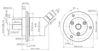
Order example for 10 mm shaft diameter: AHx36I-SCxx0xxxxx + BEF-FA-020-036-I (adapter is not pre-assembled)
