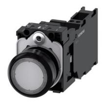
Illuminated pushbutton, 22 mm, round, plastic, clear, pushbutton, flat, momentary contact type, with holder, 1 NO+1 NC, LED module with integrated LED 230 V AC, spring-type terminal, with laser labeling, inscription or symbol Customer-specific selection with SIRIUS ACT configurator (CIN)
