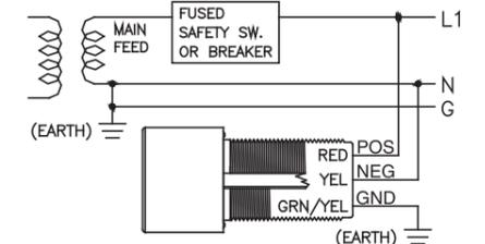
**R-3D2 WIRING CONFIGURATIONS**
