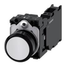
Pushbutton, 22 mm, round, plastic, white, pushbutton, flat, momentary contact type, with holder 1 NO+1 NC, spring-type terminal, with laser labeling, upper case and lower case, always upper case at the beginning of the word
